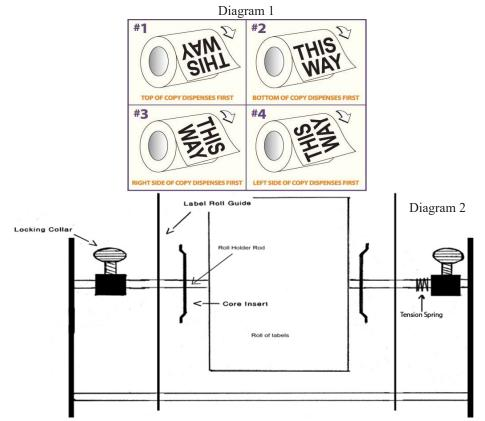
There are two 9" long, metal roll guides and a tension spring included with the machine. These guides should be placed on either side of the roll of labels between the metal core inserts and the locking collar. The notches on the end of the guide slide onto the chrome rod at the bottom of the machine. Tension spring goes between the right roll guide and the locking collar on the right side of the roll of labels as shown in diagram 2.
